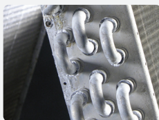
Aluminum tube and tube sheet after 500 hour salt spray.
